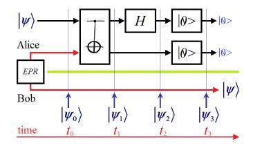
Figure 30 Controlled quantum teleportation protocol.
