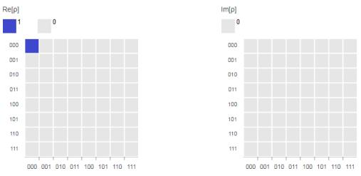
Figure 59 Wavefunction's density matrix: on the left, the real part, and on the right, the imaginary part.
