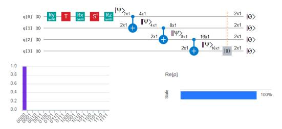
**Figure 77** On the top, the generation of a not maximally entangled pair, then, two successive *CNOT* gates appear in cascade. The presence of a qubit reset gate [|0>] in the lowest branch simultaneously produces an automatic collapse of all the outputs to the ground state |0>, destroying the stretching and the quasi-entanglement. Finally, the bottom-left, shows a unitary wavefunction's complex modulus, while, bottom-right, shows the real part of the state, which is unitary too.
