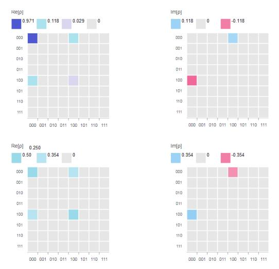
Figure 57 Top: wavefunction's density matrix for the first type of statevector, and, bottom: wavefunction's density matrix for the second type of statevector delivered by IBM Q [42].
