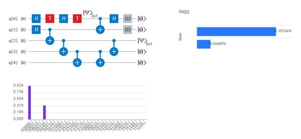
**Figure 71** On the top-left is the quantum circuit for controlled quantum teleportation where the lower branch of the EPR pair is stretched twice and shrunk twice, annulling their effects mutually. On the bottom-left, the height of the bar is the complex modulus of the wavefunction. Finally, on the right is the real part of the state.
