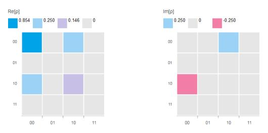
Figure 21 Wavefunction's density matrix: on the left, the real part, and on the right, the imaginary part.
