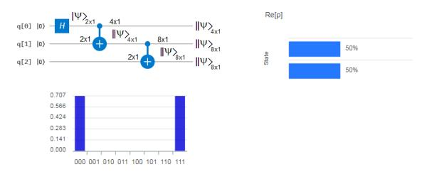
**Figure 24** On the top-left is the quantum circuit for multiple entanglement generation thanks to two *CNOT* gates in cascade which produces three wavefunctions. Before and after each *CNOT* gate we can see the size of the statevector and the wavefunctions as vectors. On the bottom-left, the height of the bar is the complex modulus of the wavefunction. Finally, on the right is the real part of the state.
