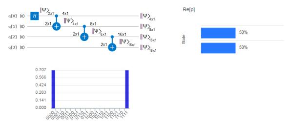
**Figure 27** On the top-left is the quantum circuit for a multiple entanglement generation thanks to three *CNOT* gates in cascade, which produces four wavefunctions. Before and after each *CNOT* gate, we can see the size of the statevector and the wavefunctions as vectors. On the bottom-left, the height of the bar is the complex modulus of the wavefunction. Finally, on the right is the real part of the state.
