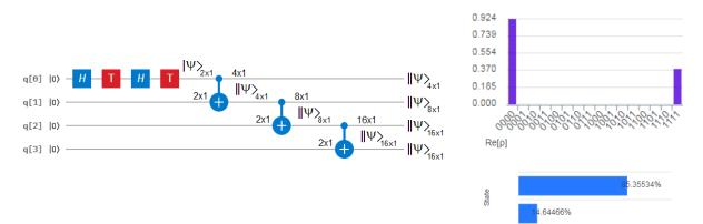
**Figure 7** On the left is the quantum circuit for the qubit generation and the cascade of *CNOT* gates with four outcomes of different sizes. Before and after each *CNOT* gate we can see the size of the statevector and the wavefunctions as vectors. On the upper-right, the height of the bar is the complex modulus of the wavefunction. Finally, on the lower-right is the real part of the state.
