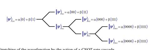
Figure 8 Stretching of the wavefunction by the action of a CNOT gate cascade.
