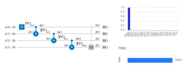
**Figure 75** On the left, the configuration starts with the generation of the |+> state, the first *CNOT* gate generates an EPR pair, while the following ones produce successive stretchings of the pair. The qubit reset gate in the lowest branch put all the output to ground state |0>. On the top-right is the unitary wavefunction's complex modulus, and on the bottom-right is the real part of the state, which is unitary too.
