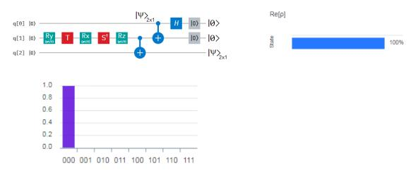
**Figure 58** On the top-left is the quantum circuit for controlled quantum teleportation of  $|0\rangle$  via a not maximally entangled pair. On the bottom-left, the height of the bar is the complex modulus of the wavefunction. Finally, on the right is the real part of the state.
