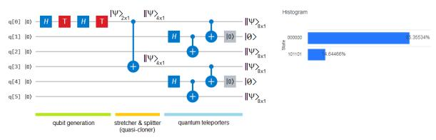
Figure 91 Identical considerations about the previous cases, however, the use of a simplified version of the teleporters generates more stretching at the output of the configuration.
