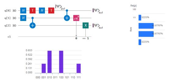
**Figure 37** On the top-left is the quantum circuit for simplified and uncontrolled quantum teleportation. On the bottom-left, the height of the bar is the complex modulus of the wavefunction. Finally, on the right is the real part of the state.
