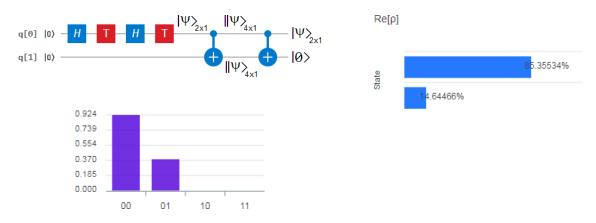
**Figure 18** On the top-left is the quantum circuit for the qubit generation and the cascade of two *CNOT* gates with two outcomes: the original state and the ground state. Before and after each *CNOT* gate we can see the size of the statevector and the wavefunctions as vectors. On the bottom-left, the height of the bar is the complex modulus of the wavefunction. Finally, on the right is the real part of the state.
