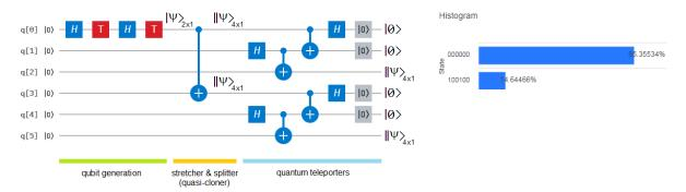
**Figure 89** On the left, the quantum circuit for this experiment begins with the qubit generation, and continues with a quantum stretching, where each branch goes to its respective teleporter. On the right, the histogram with the real part of the state.
