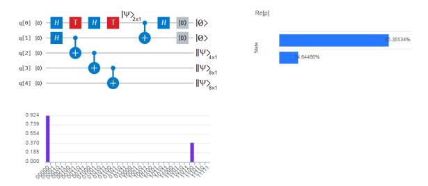
**Figure 67** On the top-left is the quantum circuit for controlled quantum teleportation where the lower branch of the EPR pair is stretched allowing another receiver additional to Bob. On the bottom-left, the height of the bar is the complex modulus of the wavefunction. Finally, on the right is the real part of the state.
