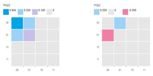
Figure 19 Wavefunction's density matrix: on the left, the real part, and on the right, the imaginary part.
