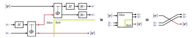
Figure 62 The controlled quantum teleportation ends up in a big SWAP or cross.
