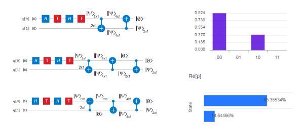
**Figure 20** On the left are three quantum circuit to provoke a *SWAP* action. On the top-right, the height of the bar is the complex modulus of the wavefunction, which, in this case, also coincides with the wavefunction itself. Finally, on the bottom-right is the real part of the state.
