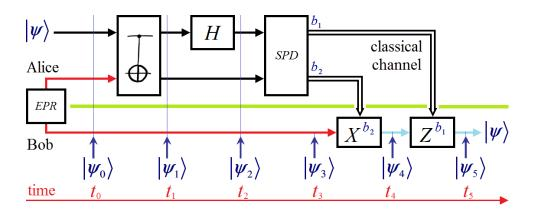
**Figure 29** Uncontrolled (original) quantum teleportation. EPR means EPR pair generation procedure, X and Z are the corresponding Pauli's matrices, H is a Hadamard's gate, SPD is the *single-photon detector* module, while,  $b_1$  and  $b_2$  are the classical bits of disambiguation that travel via the classical channel from Alice to Bob.
