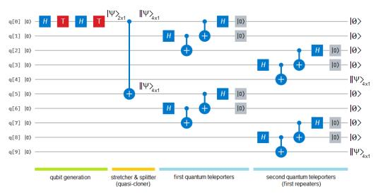
Figure 94 Complete configuration with qubit generation, quantum stretching, two lines of teleporters: the first line and their respective repeaters, i.e., the second line.
