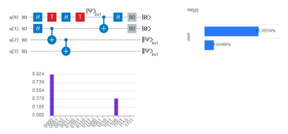
**Figure 64** On the top-left is the quantum circuit for controlled quantum teleportation where the lower branch of the EPR pair is stretched allowing another receiver additional to Bob. On the bottom-left, the height of the bar is the complex modulus of the wavefunction. Finally, on the right is the real part of the state.
