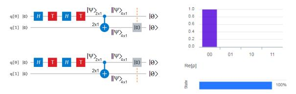
**Figure 73** On the left, both versions for a blocking via qubit reset gate in one of the two branches at the output of the *CNOT* gate. On the top-right is the unitary wavefunction's complex modulus, and on the bottom-right is the real part of the state, which is unitary too.
