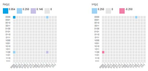
Figure 65 Wavefunction's density matrix: on the left, the real part, and on the right, the imaginary part.
