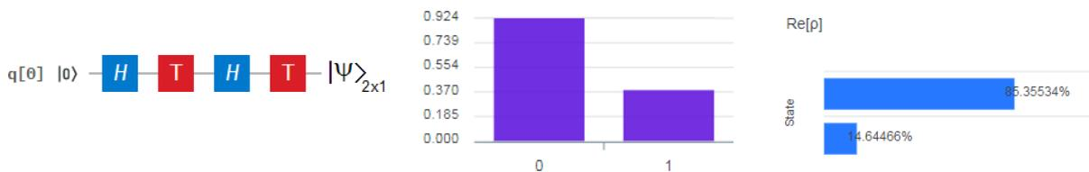
**Figure 2** On the left is the quantum circuit for the qubit generation. In the middle, the height of the bar is the complex modulus of the wavefunction. Finally, on the right is the real part of the state.
