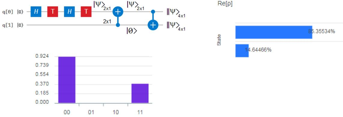
**Figure 22** On the top-left is the quantum circuit for the qubit generation and the cascade of two *CNOT* gates in opposition with two outcomes: both stretched. Before and after each *CNOT* gate we can see the size of the statevector and the wavefunctions as vectors. On the bottom-left, the height of the bar is the complex modulus of the wavefunction. Finally, on the right is the real part of the state.
