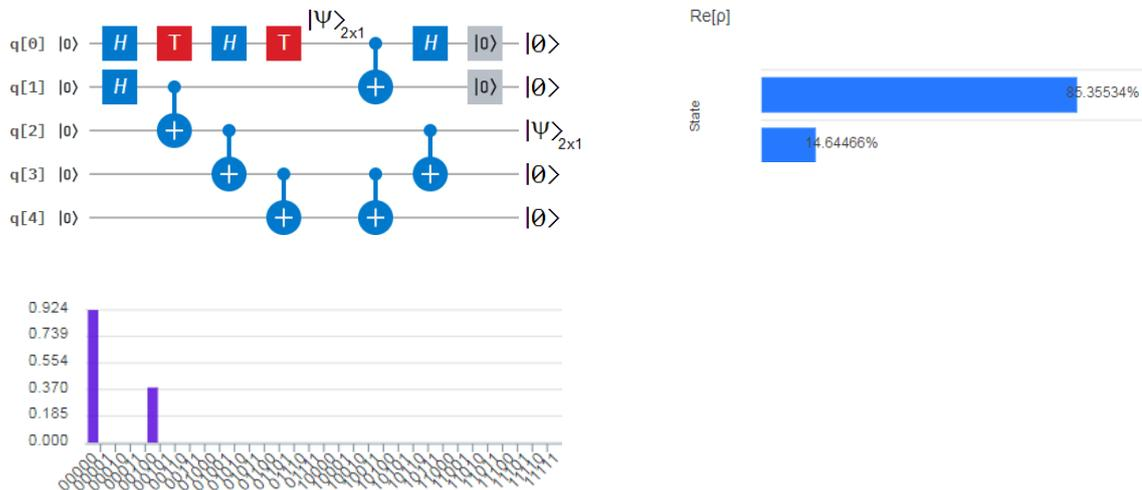
**Figure 71** On the top-left is the quantum circuit for controlled quantum teleportation where the lower branch of the EPR pair is stretched twice and shrunk twice, annulling their effects mutually. On the bottom-left, the height of the bar is the complex modulus of the wavefunction. Finally, on the right is the real part of the state.
