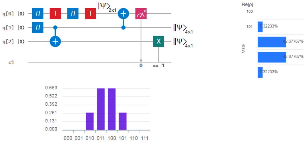
**Figure 39** On the top-left is the quantum circuit for simplified and uncontrolled quantum teleportation. On the bottom-left, the height of the bar is the complex modulus of the wavefunction. Finally, on the right is the real part of the state.
