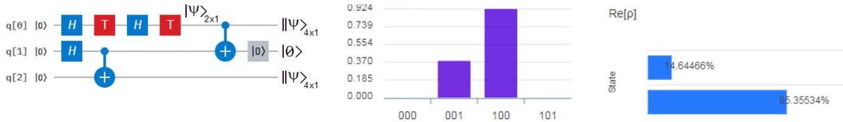
**Figure 45** On the left is the quantum circuit for the qubit generation in q[0] and the simplified *BSC* in q[0] and q[1]. In the middle, the height of the bar is the complex modulus of the wavefunction. On the right is the real part of the state (histogram o measurement probabilities).
