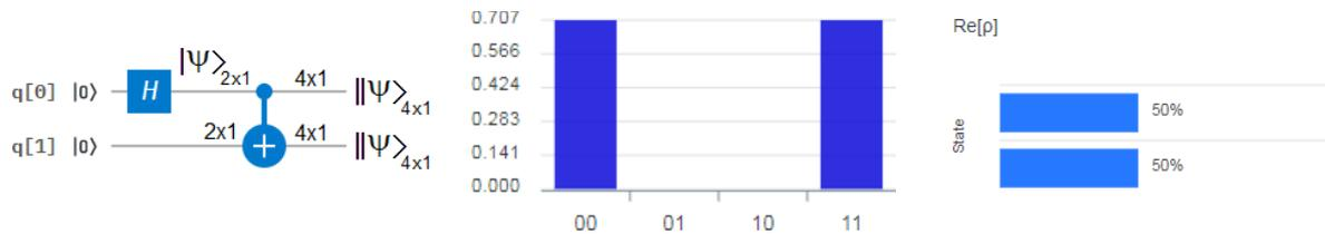
**Figure 12** The quantum circuit for the qubit generation and *CNOT* gate which causes quasi-copy and stretching is on the left. In the middle, the height of the bar is the complex modulus of the wavefunction, which, in this case, also coincides with the wavefunction itself. Finally, the real part of the state is on the right.
