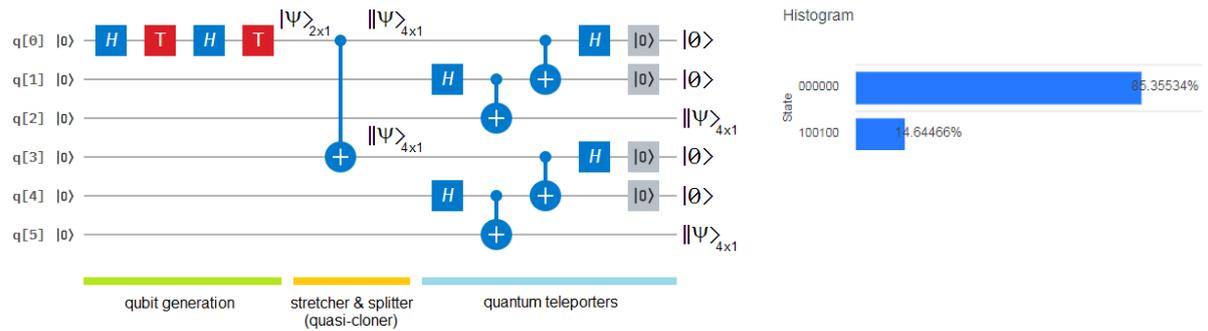
**Figure 89** On the left, the quantum circuit for this experiment begins with the qubit generation, and continues with a quantum stretching, where each branch goes to its respective teleporter. On the right, the histogram with the real part of the state.
