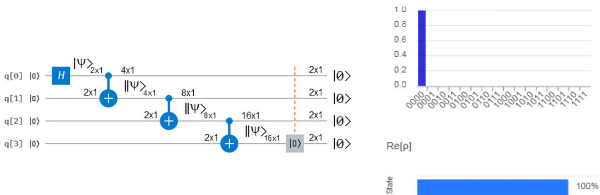
**Figure 75** On the left, the configuration starts with the generation of the  $|+\rangle$  state, the first *CNOT* gate generates an EPR pair, while the following ones produce successive stretchings of the pair. The qubit reset gate in the lowest branch put all the output to ground state  $|0\rangle$ . On the top-right is the unitary wavefunction's complex modulus, and on the bottom-right is the real part of the state, which is unitary too.
