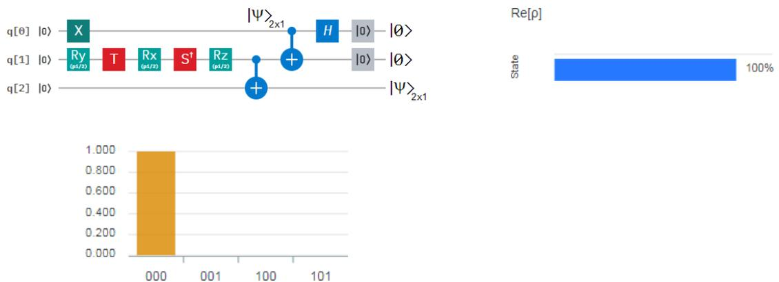
**Figure 60** On the top-left is the quantum circuit for controlled quantum teleportation of  $|1\rangle$  via a not maximally entangled pair. On the bottom-left, the height of the bar is the complex modulus of the wavefunction. Finally, on the right is the real part of the state.
