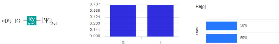
**Figure 49** On the left is the quantum circuit for the qubit generation in q[0]. In the middle, the height of the bar is the complex modulus of the wavefunction, which is typical of a  $|+\rangle$  state. On the right is the real part of the state, also typical of a  $|+\rangle$  state.
