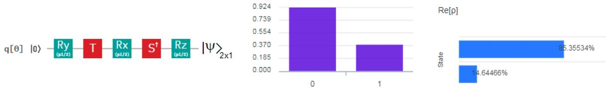
**Figure 53** On the left is the quantum circuit for the qubit generation in q[0]. In the middle, the height of the bar is the complex modulus of the wavefunction, which is different from that of **Figure 49**. On the right is the real part of the state, also it is different from that of **Figure 49**.
