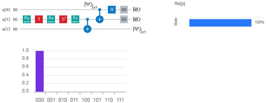
**Figure 58** On the top-left is the quantum circuit for controlled quantum teleportation of  $|0\rangle$  via a not maximally entangled pair. On the bottom-left, the height of the bar is the complex modulus of the wavefunction. Finally, on the right is the real part of the state.
