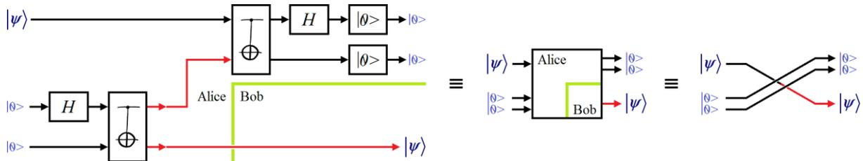
**Figure 62** The controlled quantum teleportation ends up in a big *SWAP* or cross.
