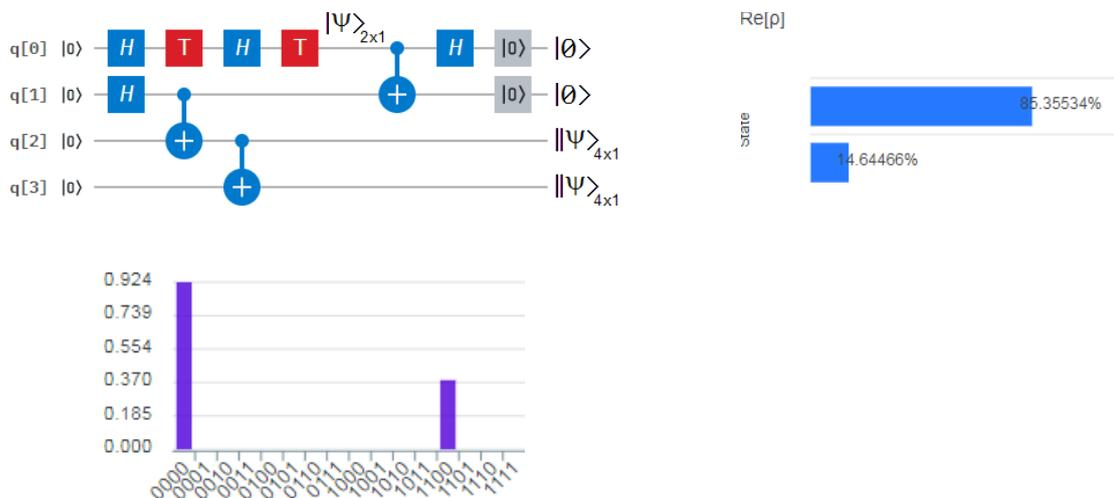
**Figure 64** On the top-left is the quantum circuit for controlled quantum teleportation where the lower branch of the EPR pair is stretched allowing another receiver additional to Bob. On the bottom-left, the height of the bar is the complex modulus of the wavefunction. Finally, on the right is the real part of the state.
