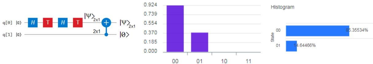
**Figure 16** On the left is the quantum circuit for the qubit generation and a *CNOT* gate from q[1] to q[0]. In the middle, the height of the bar is the complex modulus of the wavefunction, which, in this case, also coincides with the wavefunction itself. On the right is the real part of the state (histogram of measurement probabilities).
