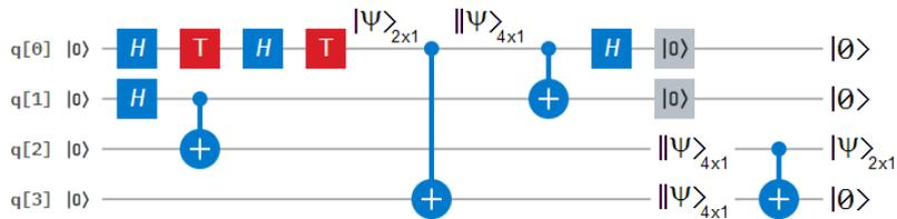
**Figure 86** With a similar scheme to the previous case, the final *CNOT* gate at the output between qubits q[2] and q[3] restores the original qubit to be teleported, without the need to measure it so as not to alter it, instead, we measure q[3] and depending on how similar it is to a  $|0\rangle$ , it indirectly but with total accuracy that we evaluate the quality of teleportation.
