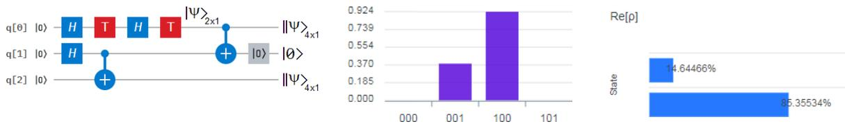
**Figure 45** On the left is the quantum circuit for the qubit generation in q[0] and the simplified BSC in q[0] and q[1]. In the middle, the height of the bar is the complex modulus of the wavefunction. On the right is the real part of the state (histogram o measurement probabilities).
