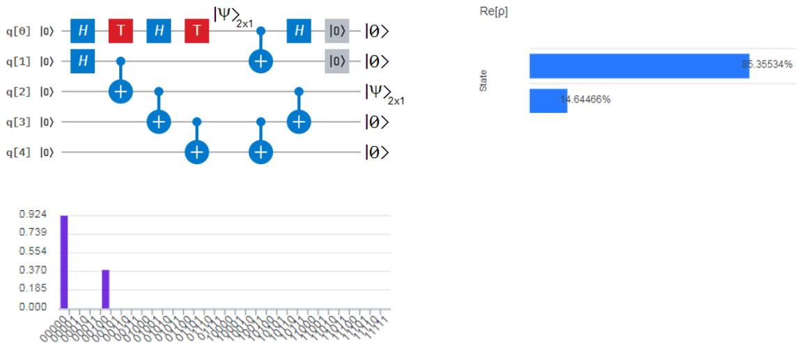
**Figure 71** On the top-left is the quantum circuit for controlled quantum teleportation where the lower branch of the EPR pair is stretched twice and shrunk twice, annull their effects mutually. On the bottom-left, the height of the bar is the complex modulus of the wavefunction. Finally, on the right is the real part of the state.
