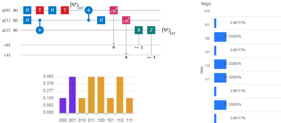
**Figure 35** On the top-left is the quantum circuit for robust and uncontrolled quantum teleportation. On the bottom-left, the height of the bar is the complex modulus of the wavefunction. Finally, on the right is the real part of the state.
