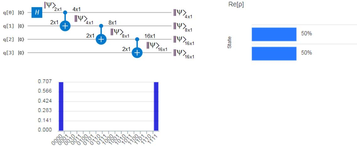
**Figure 27** On the top-left is the quantum circuit for a multiple entanglement generation thanks to three *CNOT* gates in cascade, which produces four wavefunctions. Before and after each *CNOT* gate, we can see the size of the statevector and the wavefunctions as vectors. On the bottom-left, the height of the bar is the complex modulus of the wavefunction. Finally, on the right is the real part of the state.
