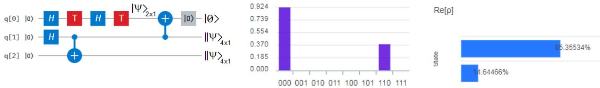
**Figure 47** On the left is the quantum circuit for the qubit generation in q[0] and the swapped simplified BSC in q[1] and q[0]. In the middle, the height of the bar is the complex modulus of the wavefunction. On the right is the real part of the state (histogram o measurement probabilities).
