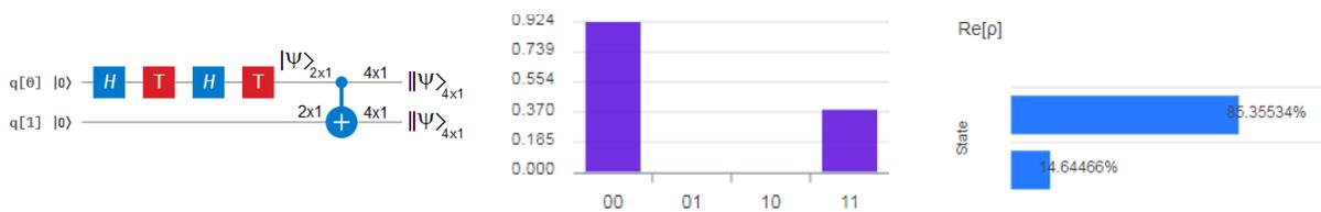
**Figure 4** On the left is the quantum circuit for the qubit generation and *CNOT* gate which causes quasi-copy and stretching. In the middle, the height of the bar is the complex modulus of the wavefunction. Finally, on the right is the real part of the state.
