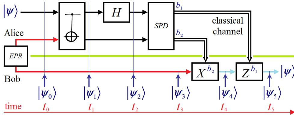
**Figure 29** Uncontrolled (original) quantum teleportation. EPR means EPR pair generation procedure, X and Z are the corresponding Pauli's matrices, H is a Hadamard's gate, SPD is the *single-photon detector* module, while,  $b_1$  and  $b_2$  are the classical bits of disambiguation that travel via the classical channel from Alice to Bob.
