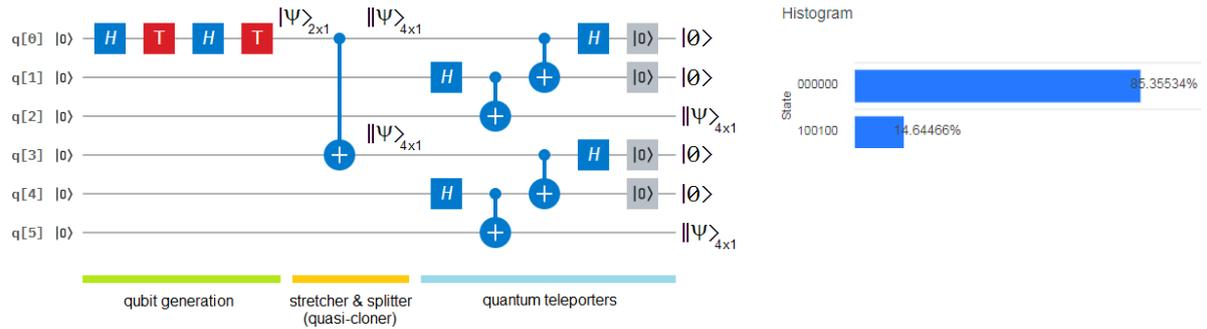
**Figure 89** On the left, the quantum circuit for this experiment, which begins with the qubit generation, continue with a quantum stretching where each branch go to its respective teleporter. On the right, the histogram with the real part of the state.
