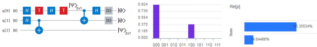
**Figure 41** On the left is the quantum circuit for the qubit generation in  $q[0]$  and the BSC in  $q[0]$  and  $q[1]$ . In the middle, the height of the bar is the complex modulus of the wavefunction. On the right is the real part of the state (histogram o measurement probabilities).
