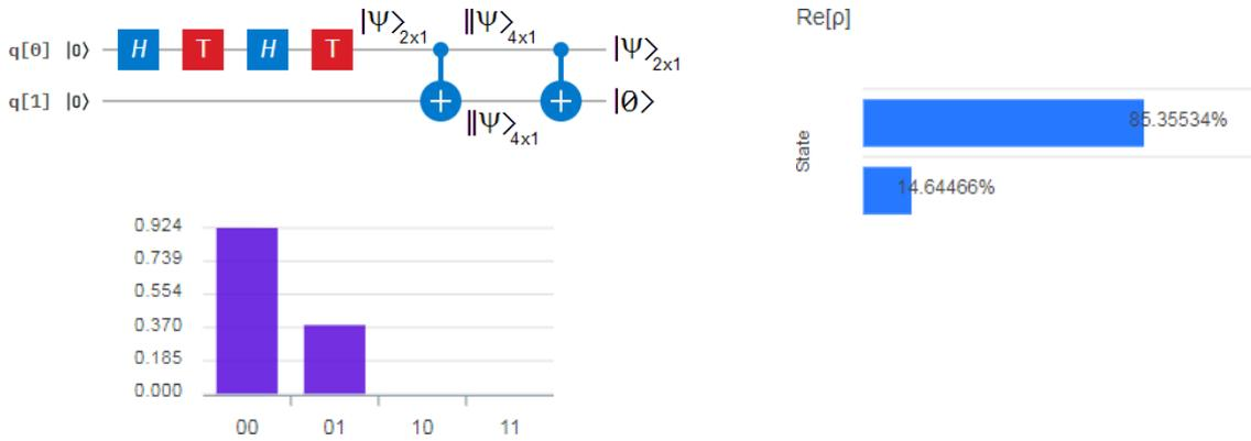
**Figure 18** On the top-left is the quantum circuit for the qubit generation and the cascade of two *CNOT* gates with two outcomes: the original state and the ground state. Before and after each *CNOT* gate we can see the size of the statevector and the wavefunctions as vectors. On the bottom-left, the height of the bar is the complex modulus of the wavefunction. Finally, on the right is the real part of the state.
