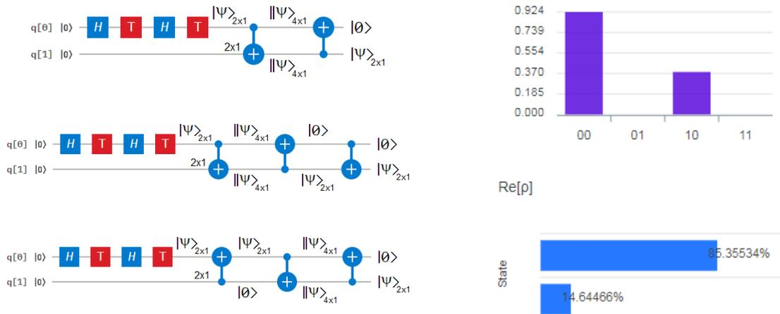
**Figure 20** On the left are three quantum circuit to provoke a *SWAP* action. On the top-right, the height of the bar is the complex modulus of the wavefunction, which, in this case, also coincides with the wavefunction itself. Finally, on the bottom-right is the real part of the state.
