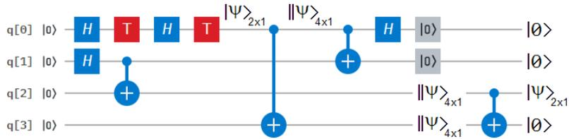
**Figure 86** With a similar scheme to the previous case, the final *CNOT* gate at the output between qubits  $q[2]$  and  $q[3]$  restores the original qubit to be teleported, and without the need to measure it so as not to alter it, instead, we measure  $q[3]$  and depending on how similar it is to a  $|0\rangle$ , it is indirectly but with total accuracy that we evaluate the quality of teleportation.
