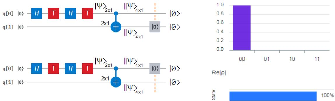
**Figure 73** On the left, both versions for a blocking via qubit reset gate in one of the two branches at the output of the *CNOT* gate. On the top-right is the unitary wavefunction's complex modulus, and on the bottom-right is the real part of the state, which is unitary too.
