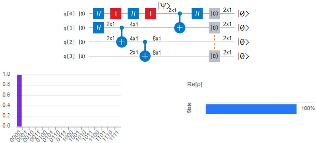
**Figure 79** On the top, a controlled quantum teleportation protocol with stretching on the lowest branch of the EPR pair generation module with blocking on one of its two stretched branches. The bottom-left shows a unitary wavefunction's complex modulus. The bottom-right shows the real part of the state, which is unitary too.
