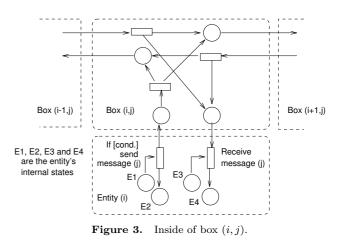
Such a virtual medium liking n entities that is capable of exchanging m different sorts of messages, consists of m lines like those shown in figure 2. Hence, the medium's complexity does not depend on the number of communicating entities. The drawback with such a medium is that receivers of a message do not get it simultaneously. However, this is no problem when modeling asynchronous interactions.
