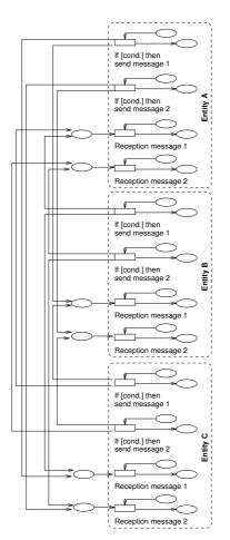
Figure 1. Perfect virtual medium linking three communicating entities, and allowing the exchange of two types of messages.
