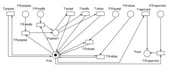
Figure 5. Petri sub-net modeling an agent that makes use of the negotiation protocol seen in figure 4.
