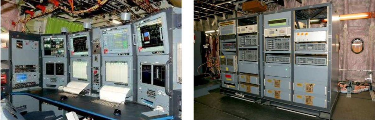
Figure 1: Flight Test Engineer Station and associated servers for A380 (2005)
