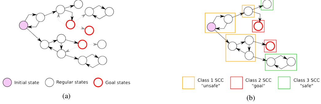
FIGURE 2 – Attack Graph generation algorithm : (a) the transition function is restricted to non-goal states, and (b) construction of the SCC graph using Tarjan’s algorithm and partitioning of the set of components into three mutually exclusive classes.
