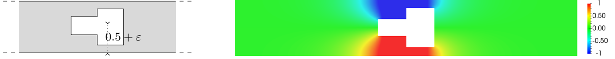
Figure 5: Left: geometry of \Omega^\varepsilon . Right: real part of a trapped mode for \varepsilon = 0 and \sqrt{\lambda^0} \approx 1.9939 .
