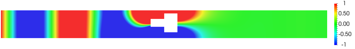
Figure 8: Real part of u_+ in \Omega^\varepsilon for \varepsilon = 0.05 and \sqrt{\lambda} = 2.0072 . In this setting, we have T(\varepsilon, \lambda) \approx 0 .
