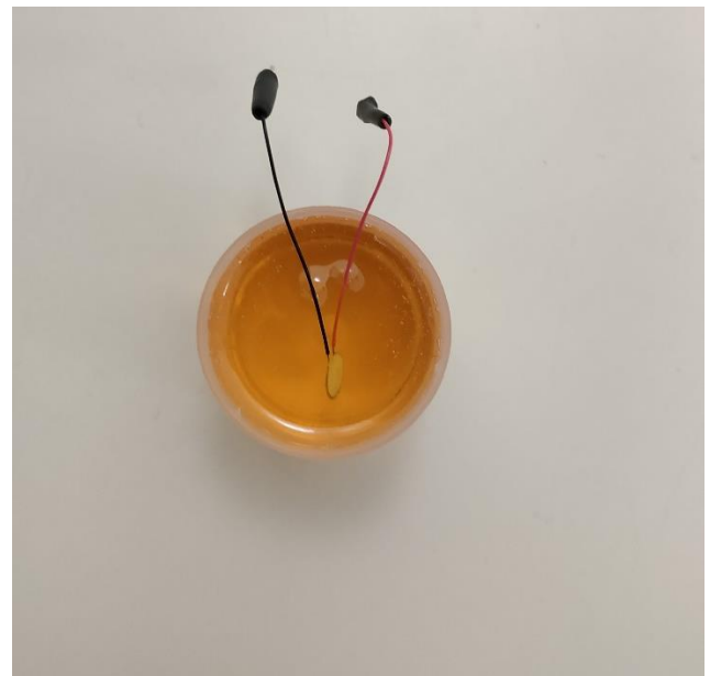
Fig. 3. Specimen of epoxy resin curing monitoring
