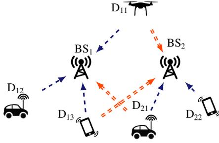
Fig. 1. System composed of five mobile devices ( $D_{11}$ ,  $D_{12}$ , etc.) and two base stations ( $BS_1$ ,  $BS_2$ ). The blue arrows represent the direct links while the red (double-lined) ones are interfering links.
