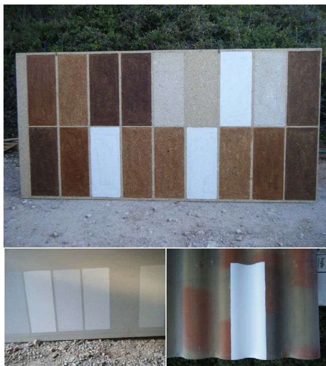
Figure 1: Paints and varnishes with ENPs additives, and paints containing ENPs on wood panel (top), plaster with cardboard (bottom left) and cement plate (bottom right).
