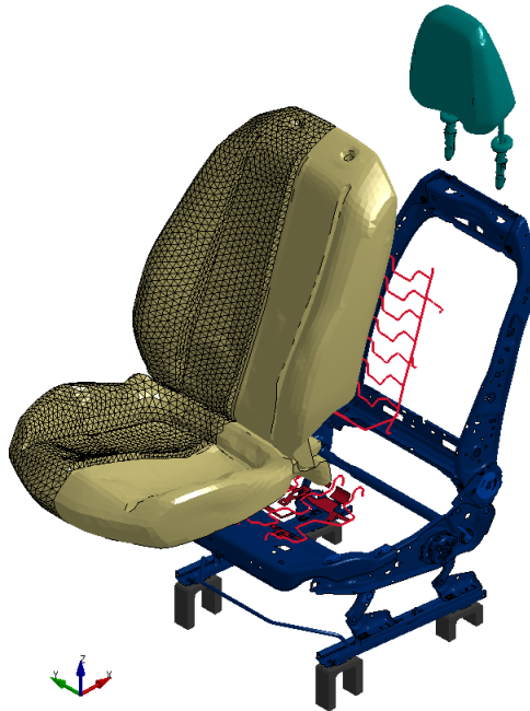
Figure 3: Exploded view of the complete seat finite element model.
