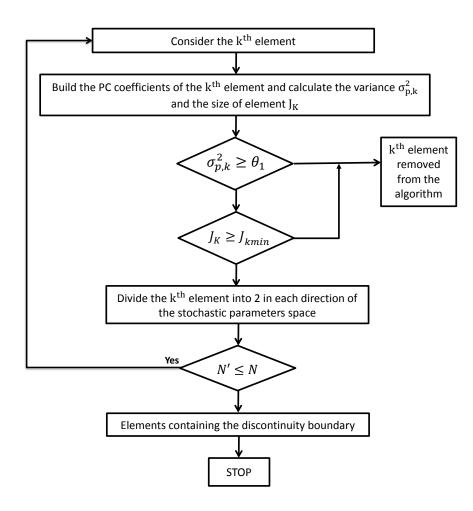
Figure 5: Algorithm of the ME-gPC based method to identify the mitigation limit.
