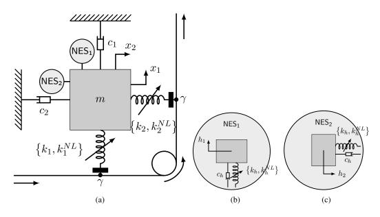
Figure 1: (a) Mechanical system with NESs. (b) Zoom on the NES<sub>1</sub>. (c) Zoom on the NES<sub>2</sub>.
