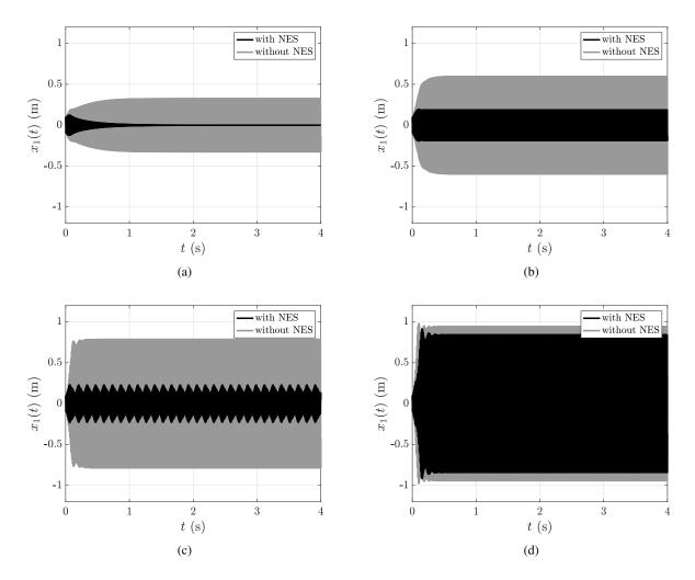
Figure 3: Comparison between time serie  $x_1(t)$  resulting from the numerical integration of the braking system with and without NESs. (a) Complete suppression,  $\gamma = 0.16$ ; (b) Mitigation: PR,  $\gamma = 0.18$ ; (c) Mitigation: SMR,  $\gamma = 0.2$ ; (d) No suppression,  $\gamma = 0.22$ . The set of parameters Eq. (2) is used.
