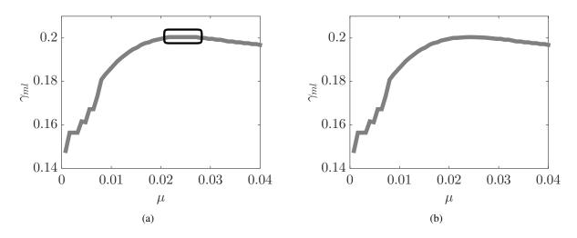
Figure 6: Variation of the mitigation limit as a function of the damping ratio of the NES ( $\mu$ ) by the deterministic method. (a) 50 samples of  $\mu \in [0, 0.04]$ ; (b) 10 added samples of  $\mu \in [0.02, 0.03]$ .
