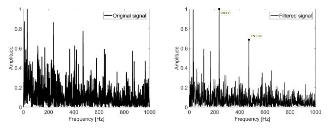
Figure 6: Experimental case: (Left) The envelope spectrum of the raw input signal. (Right) The envelope spectrum after filtering with the proposed LPE method.
