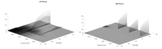
Figure 4: Squared envelope spectrum waterfall plot after filtering with the proposed method based on the relter filtering with the MED method based on kurtosis.
