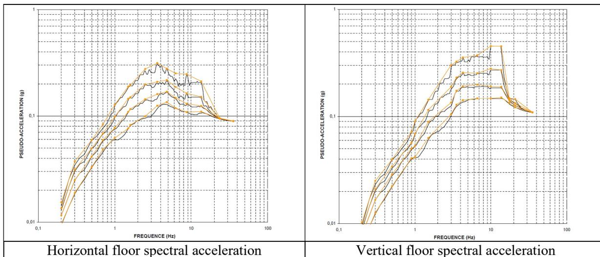
Figure 1: Horizontal and vertical floor spectral accelerations
