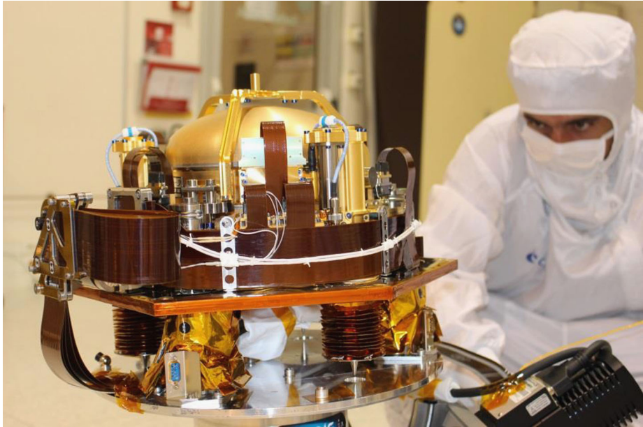
Fig. 11 SEIS Sensor Assembly (SA) without the RWEB
