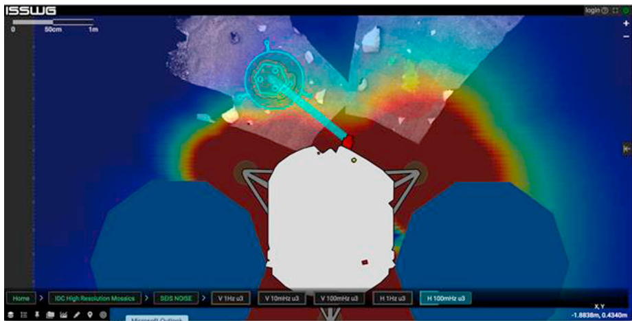
Fig. 27 This figure presents the online tool developed by JPL/Caltech to evaluate and compare the performance of tentative deployment sites. The lander is represented in the lower part of the figure. Tentative positions for SEIS (pentagon) and WTS (circle) are figured on the top. The color code goes from blue to red. It represents the percentage of budget allocation for the wind noise on the overall instrument (red equal or superior to 100, deep blue zero percent of the allocation) for the 100 mHz horizontal noise
