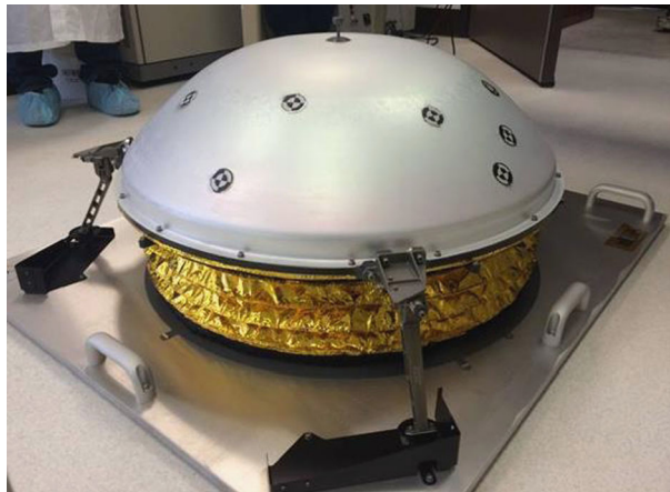
Fig. 69 SEIS RWEB (Remote Warm Enclosure Box). The width of the RWEB is \sim 355 mm and its height is 212.5 mm
