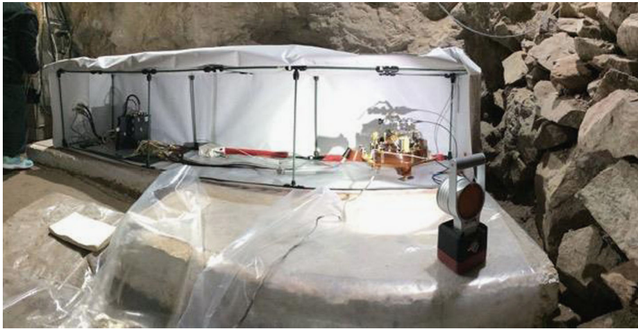
Fig. 80 Setup for SEIS QM test in the Black Forest Observatory mine seismic vault. EBOX on the left, sensor assembly with “cuvinette” on the right. Once the tent was closed the reference seismometers were installed on the pillar in the foreground
