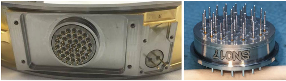
Fig. 71 (Left) 37-pin and 2-pin electrical feedthrough installed into EC Crown; (Right) 37-pin feedthrough closeup
