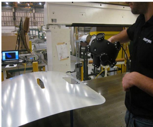
Fig 2: the handheld optical 3D Scanner “MetraSCAN” from Creafom was used to generate the SCAN mesh
