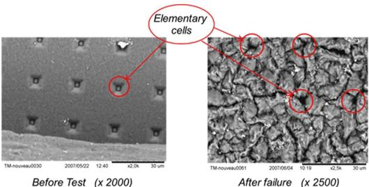
Figure 2. Topside metallization: before and after aging.
