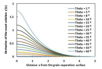
**Figure 11.** Evolution of the derivative y'(x) of the grain groove profile of the exact solution as a function of the distance x from the grain separation surface for various groove angles  $\theta$ . (*Ct* = 1).
