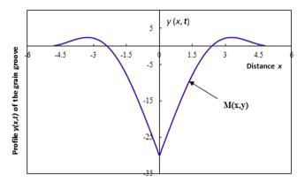
**Figure 4.** Profile y(x, t) of the grain boundary groove.
