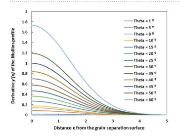
**Figure 6.** Evolution of the derivative y'(x) of the grain groove profile of Mullins approximation as a function of the distance x from the grain separation surface for various groove angles  $\theta$  from 1° to 60°.
