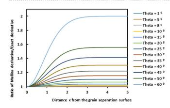
**Figure 12.** Evolution of the ratio of Mullins derivative on the exact derivative of the grain groove profile as a function of the distance *x* from the grain separation surface for different values of groove angle  $\theta$ . (*Ct* = 1).
