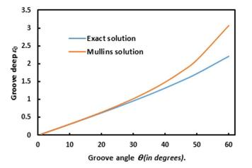
**Figure 13.** Evolution of the Groove deep  $\varepsilon_0$  as a function the groove angle  $\theta$  in two cases of Mullins solution and the exact solution.
