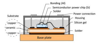
Figure 1. High power IGBT module.
