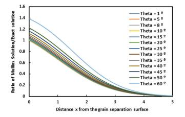
**Figure 8.** Evolution of the ratio  $(y_{Mullins}/y_{exact})$  of Mullins solution on the exact solution for the grain groove profile as a function of the distance *x* from the grain separation surface for various angles  $\theta$ . (*Ct* = 1).
