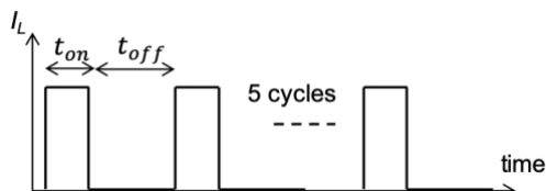
Fig. 8: Schematic load current cycles for numerical simulations.
