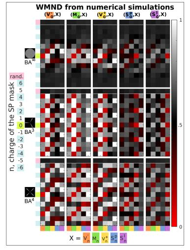
Fig. 7: Weighted Median Normalized Distance (WMND) for all possible pairs of critical points screened here, for the addition of spiral phase mask with charges up to  $n = \pm 6$  and for the apertures  $BA^N$  ( $N \in \{3, 4, \infty\}$ ). The WMND were computed from numerical simulations.
