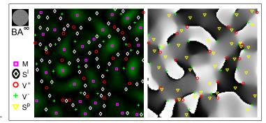
Fig. 6: Detected critical points superimposed to the filtered experimental intensity (left) and phase (right) patterns obtained with the aperture  $BA^{\infty}$ . The displayed pattern correspond to an area of  $150 \times 150$  pixels on the camera. Phase vortices ( $V^+$  and  $V^-$ ) are also zeros of the intensity pattern. Notations for the critical points are identical to those introduced in the core of the main article.
