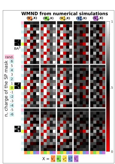
Fig. 9: Weighted Median Normalized Distance (WMND) for all possible pairs of critical points screened here, for the addition of spiral phase mask with charges up to  $n = \pm 6$  and for apertures with dihedral symmetry  $D_3$  and angular slits of width :  $\frac{\pi}{16}$ ,  $\frac{\pi}{8}$ , and  $\frac{\pi}{4}$ , respectively (from top to bottom). The WMND were computed from numerical simulations.
