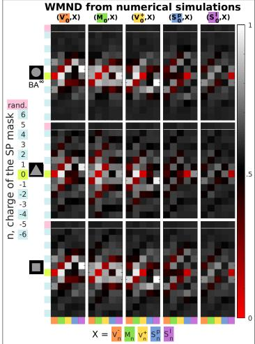
Fig. 10: WMND for all possible pairs of critical points screened here, for the addition of spiral phase mask with charges up to  $n = \pm 6$  and for a disk aperture (top) and polygonal apertures : equilateral triangle (dihedral symmetry  $D_3$ ) and square (dihedral symmetry  $D_4$ ). The WMND were computed from numerical simulations.
