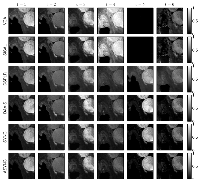
Fig. 10. Vegetation abundance map recovered by the different methods (in each row) at each time instant (given in column) for the experiment on the Mud lake data set (the different rows correspond to VCA/FCLS, SISAL/FCLS, DSPLR [5], DAVIS [21], SYNC, and ASYNC methods).
