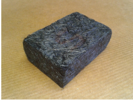
Figure 1: Entangled cross-linked fiber material: shear sample.
