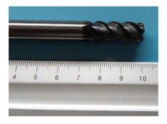
**Fig. 12.** Torus milling cutter (R = 5 r = 2).
