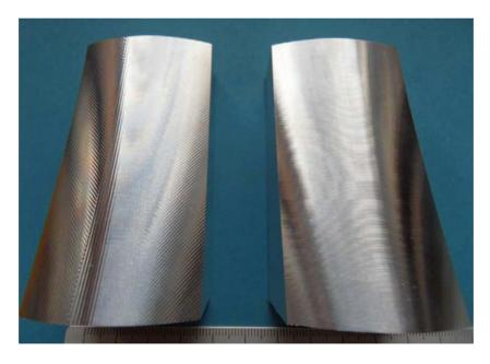
Fig. 11. Bezier surfaces machined.
