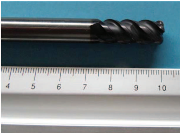
Fig. 12. Torus milling cutter ( R = 5 r = 2 ).
