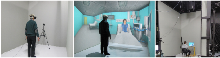
Fig. 3: Participants interacting with the virtual patient with different virtual environment displays (from left to right): virtual reality headset, virtual reality room, and PC.
