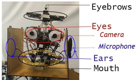
Fig. 1. Tino's head. Its eyes, composed of two pan/tilt cameras, its mouth, allowing it to display facial expressions (9 degrees of freedom) and one of its ears, created by a 3D printer and containing microphones.
