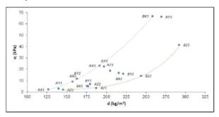
Fig. 1: Flexural strength at break of the eighteen insulation blocks, as a function of their density.
