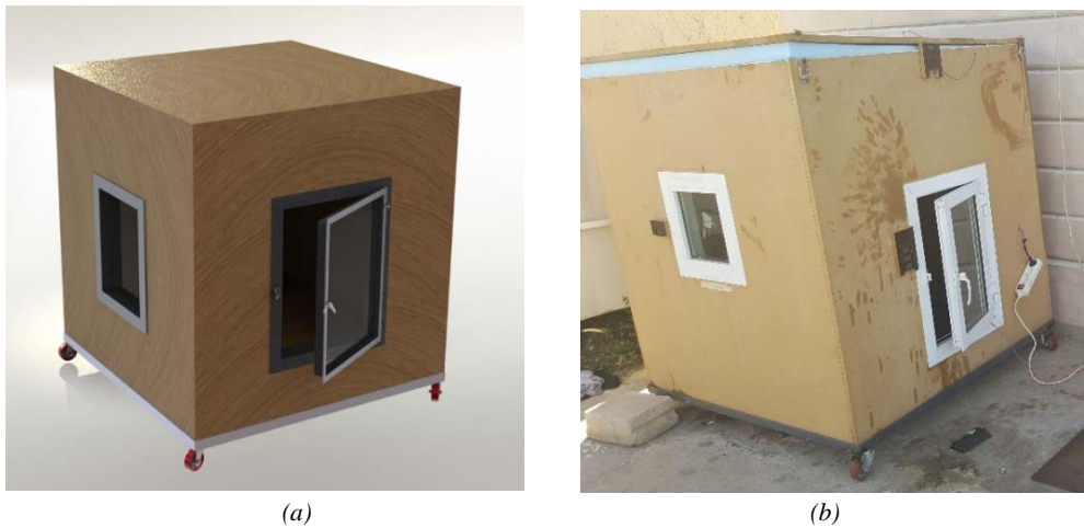
Figure 1 (a) 3D schematic drawing of the prototype, and (b) photo of the real prototype
