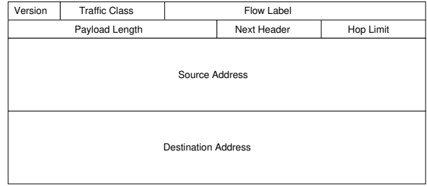
Figure 2: Standard IPv6 header.
