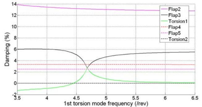
**FIGURE 6.** DAMPING FOR  $\omega_{\theta 1}$  VARIATIONS FOR A POSITIVE  $K_{45}^{\beta 3}$
