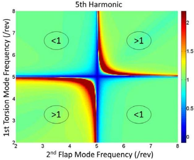
FIGURE 3. MODAL SHEAR RATIO FOR POSITIVE  $K_{45}$
