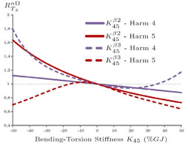
FIGURE 4. MODAL SHEAR RATIO FOR  $K_{45}^{\beta 2}$  AND  $K_{45}^{\beta 3}$
