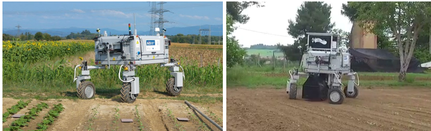
Fig. 1 These pictures show the agricultural robot BoniRob with four wheels whose orientation and rotation can be changed independently. The picture on the right has been taken during an autonomous run.
