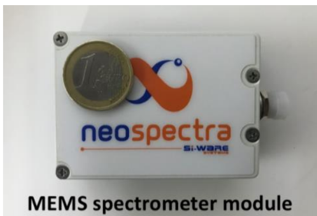
Figure 5: MEMS-based FTIR spectrometer operating in the mid-infra-red range, used to record the spectra shown in Figure 4. This suggests that the UBS-based light source can be combined with such spectrometer, for instance for chemical analysis, in an ultra-compact fashion.
