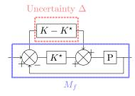
Fig. 3: Closed-loop interconnection scheme using the controller error.
