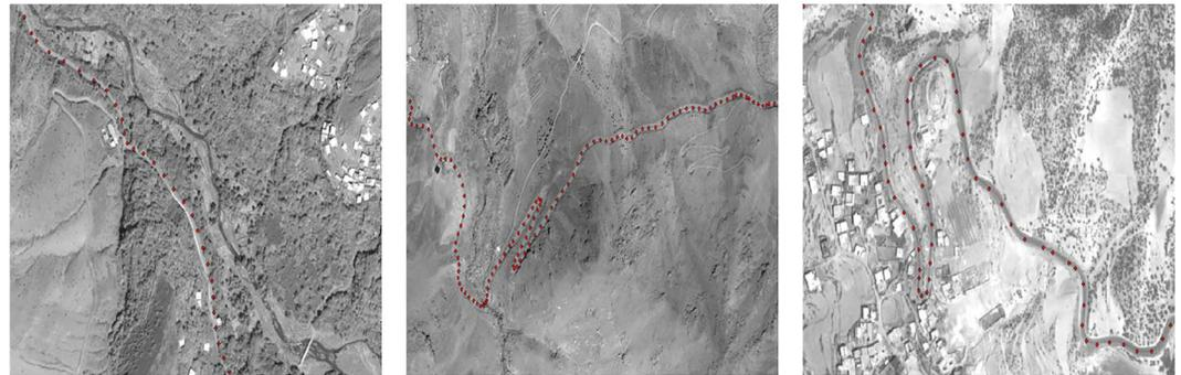
**Figure 4.** Comparison of the control points (red dots) and the orthoimage.
