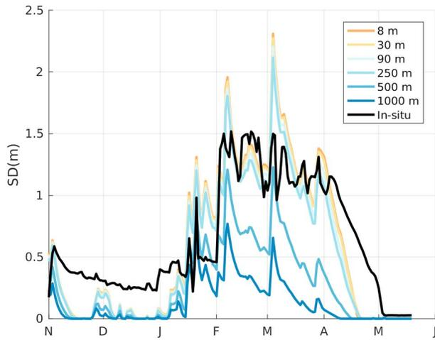
**Figure 10.** Simulated and measured snow depth at Oukaimeden (from November 2008 to June 2009) for every model resolution. SD = snow depth.
