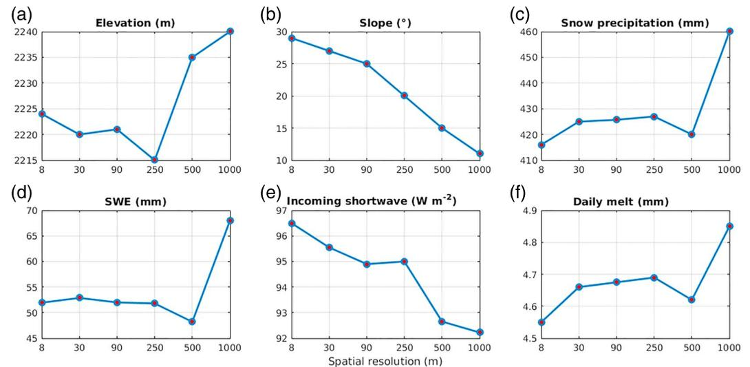
**Figure 11.** Spatial averages of (a) the model grid elevation, (b) the model grid slope, (c) the total snow precipitation, (d) the mean SWE, (e) the mean incoming shortwave radiation, and (f) the mean daily melt, for each model resolution. These values were extracted from the evaluation area, that is, the intersection of the Formosat-2 extent and the catchment area. SWE = snow water equivalent.
