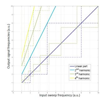
Fig. 2. Input sweep frequency versus output signal frequencies for a 4<sup>th</sup> order PHM and windowing choices examples (no overlap): linear part [optimal] (blue dashed lines), third harmonic [optimal] (green dashed lines), linear part [suboptimal] (green dot-dashed line).
