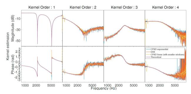
Fig. 4. PHM Kernels estimated through the classical exponential sine sweep method (ESS) and the proposed Welch Sine Sweep Method (CPSD) for two kind of sweeps versus theoretical ones in the frequency domain (SNR = 40 dB).
