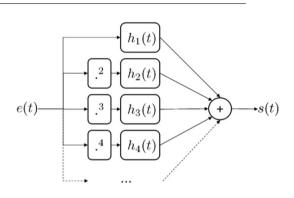
Fig. 1. Representation of parallel Hammerstein models
