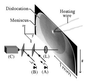
FIG. 2. Experimental setup: The vertical smectic film is observed via reflecting microscopy in monochromatic light. The objective lens (*L*) casts the image of the film on the CCD camera (*C*). The light source is the red LED (*A*). The photodiode (*B*) measures the intensity of the reflected light. The heating wire, used to nucleate the dislocation loops, is placed about 50  $\mu$ m behind the film. (The loop shown in the picture is an experimental one.)
