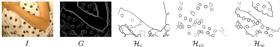
Fig. 1: An image I , the gradient G of I computed using the structured edge detector introduced in [8], the hierarchical watershed \mathcal{H}_c of G based on a regularized circularity attribute, a circularity based hierarchy \mathcal{H}_{cc} and the watershed \mathcal{H}_w of \mathcal{H}_{cc} (for G ).
