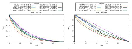
(a) Robustness in function of the per- (b) Robustness in function of the performance of studied systems for the formance of studied systems for the FVC2002 fingerprint database. POLYFKP knuckle print database.
