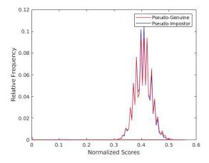
Figure 9: Pseudo-Genuine & Pseudo-Impostor distributions for unlinkability analysis. 256-bit BioCodes were generated using GREYCHashing (with C = 300 and R = 2) from 512-feature vectors, extracted with Gabor filter on the FVC2002DB1 database. Overlapped distributions indicates indistinction between BioCodes generated from the same user and BioCodes generated from the others.
