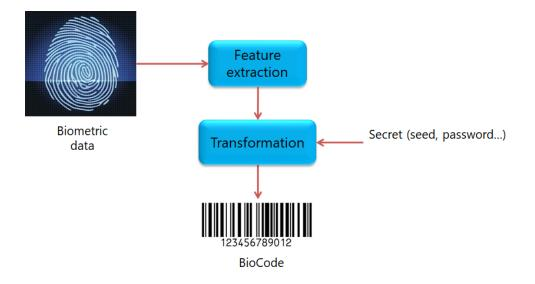
Figure 1: General principle of template protection schemes based on a transformation.
