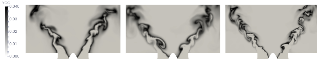
Figure 9: Instantaneous CO filtered mass fraction snapshot on the middle-plane of the combustion chamber. From left to right: AC, NAC, NAF.
