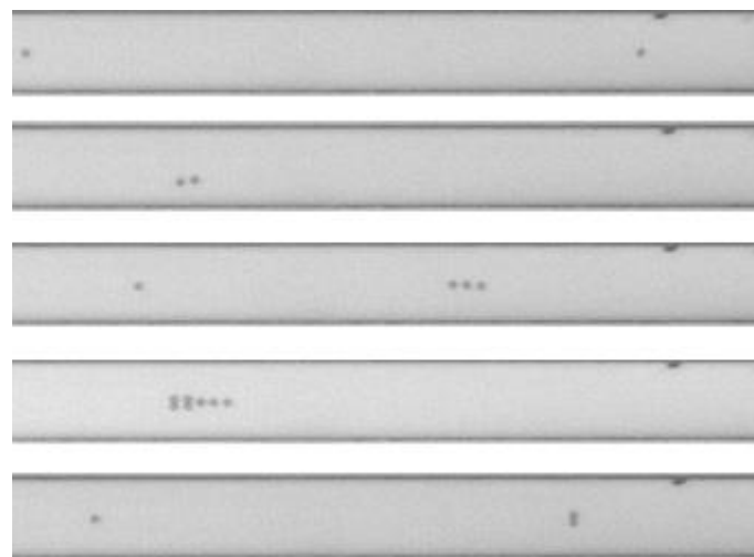
Figure S4: Observation of microdroplets at 63cm from the T-junction, for the following operational parameters: k=40 , \phi_c=0.2\mu\text{L/s} , \phi_D=0.005\mu\text{L/s} . Channel ID 150\mu\text{m} .
