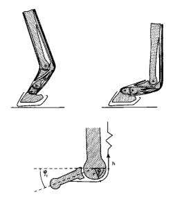
**Figure 10:** The spring construction formed by the tendon of the long finger flexor of a horse, acting around the fetlock joint. [14]
