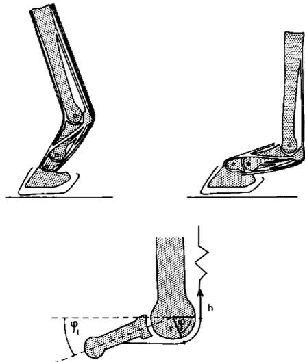
**Figure 10:** The spring construction formed by the tendon of the long finger flexor of a horse, acting around the fetlock joint. [14]
