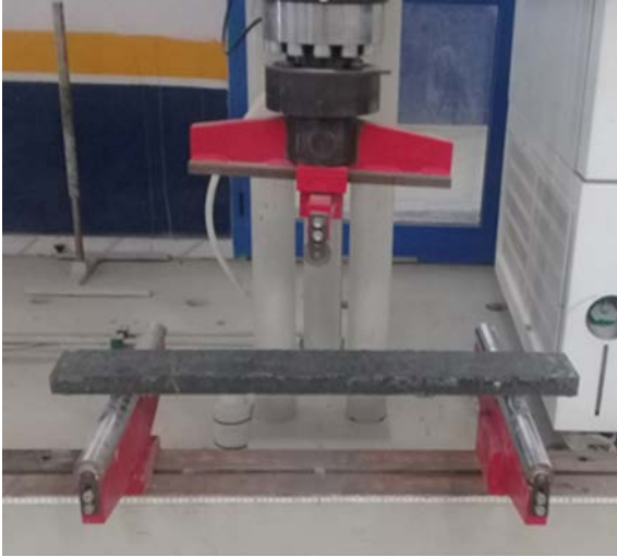
Fig. 17. Bending test set-up of the GFRC2 slab.
