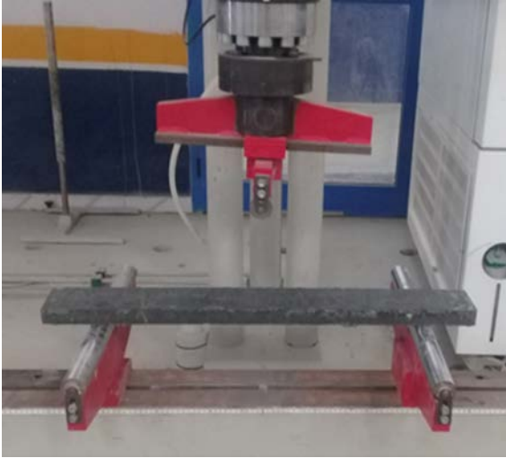
Fig. 17. Bending test set-up of the GFRC2 slab.
