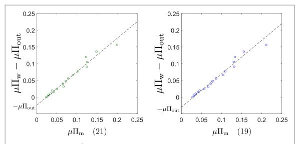
**Figure C1.**  $\mu\Pi_w - \mu\Pi_{\text{out}} = v_s \int_z^L \mathrm{d}z \rho(z)$  versus  $\mu\Pi_m$  (21) (left) and (19) (right) for experiment with  $v_s/v_0 = 0.29$ . We use this plot to measure  $\mu\Pi_{\text{out}}$  by looking at the intersect between the affine fit y = x + b and the y-axis. We find  $\mu\Pi_{\text{out}} = 0.03 \pm 0.005 \text{ s}^{-1}$  for (19), and  $\mu\Pi_{\text{out}} = 0.024 \pm 0.004 \text{ s}^{-1}$  for (21).
