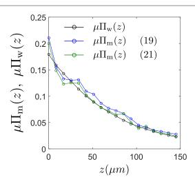
Figure 5. Pressure profiles for  $v_s/v_0=0.29$ . In black, the pressure  $\Pi_w(z)$  measured experimentally by integrating the density above a height z, following equation (22). In blue, the effective momentum flux  $\Pi_m(z)$  predicted by equation (19) and, in green, its approximation equation (21). Note that the curves for  $\Pi_m$  correspond to local measurements whereas  $\Pi_w(z)$  results from an integration. The noise level in the latter is thus much lower than in the former.
