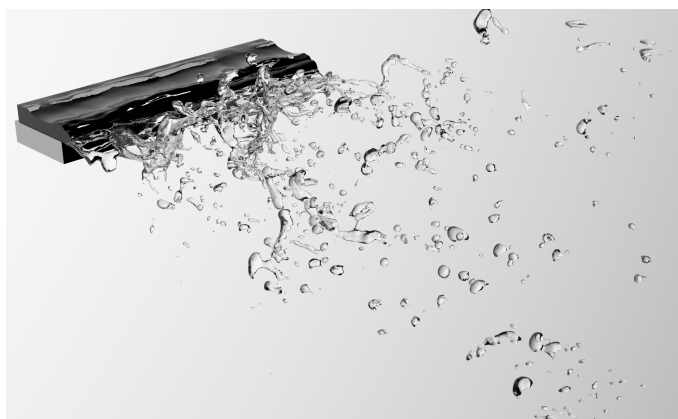
Figure 5: Rendered image displaying the formation of large number of varying sized droplets broken up from liquid sheet and ligaments.
