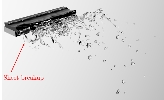
Figure 3: Liquid sheet breakup displayed in rendered image from the DNS at t = 1.51 ms. Thin sheet formation at the trailing edge of pre-filmer plate with holes subsequently breaking into small droplets of the thickness of the sheet.
