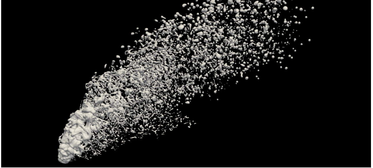
Figure 6: Visualization of liquid jet in crossflow at t^* = 32 .
