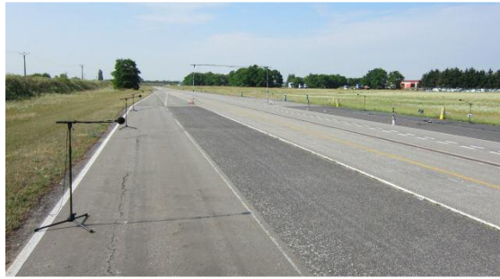
Figure 19: Measurement setup with microphones at 7.5 m
