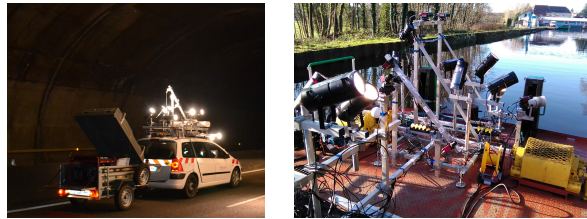
Figure 2: Imaging system mounted on a car (left) or a boat (right) for image acquisition in road or canal tunnels
